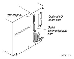
**Printer ports:** This illustration shows you where to connect your system to the printer.
